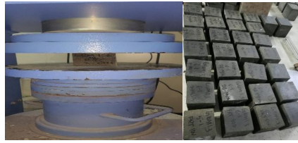
Fig. 1. Experimental setup for compressive strength testing of geo-polymer mortar cubes
