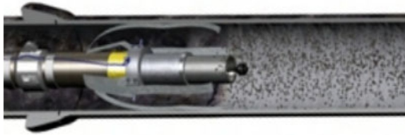
Fig. 1. Pipeline Abrasive Blasting Cleaning
