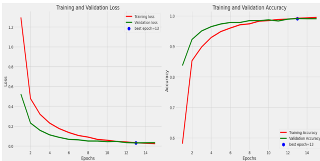
Fig. 2. Training and Validation Accuracy and Loss Curve of Fine Tuned MobileNetV2 on combined Dataset
