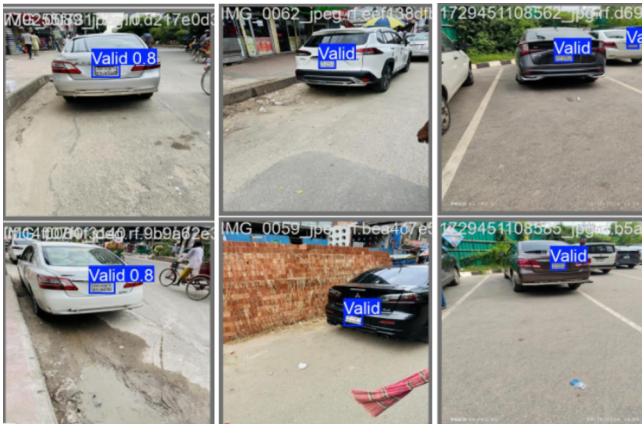
Fig. 9 License plate detection in real-time video
