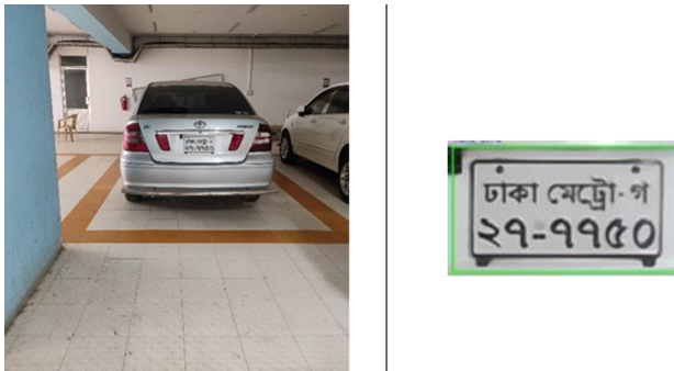
Fig. 10 Image to license plate Detection output
