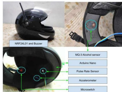
Fig. 4. Integration of main sensor modules and Control Units.
