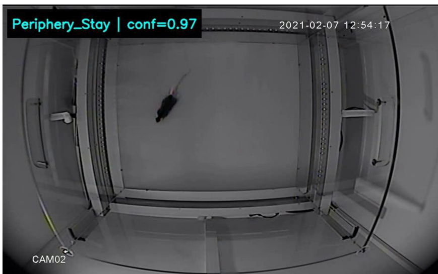
Fig. 9. Example frame from the automatically annotated Open Field Test video, showing predicted behavioral label and confidence score overlaid on the detected animal in real time.
