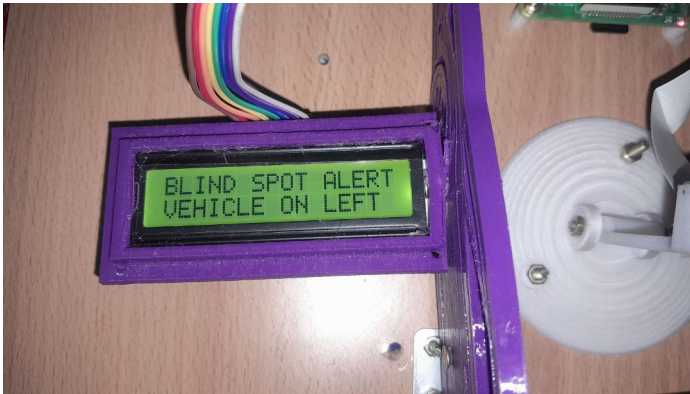
Fig. 5. Blind spot warning displayed on the LCD module during experimental testing.
