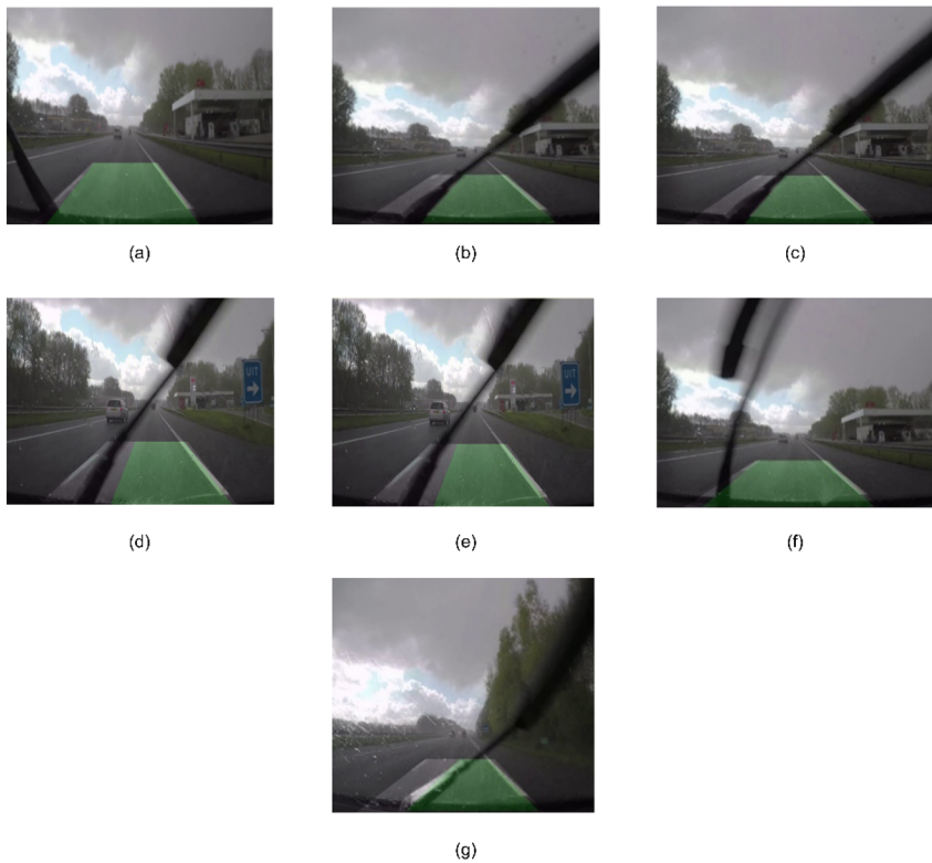
Fig. 2. (a)The frame of which the lane lines get detected correctly (b)The frame of which the wiper is wrongly detected as the lane border (c)Frame showing the edge of the wiper getting detected (d)Frame showing the edge of the wiper getting detected (e)The left lane is faded in this frame, and the edge of the wiper gets detected (f)Both the wiper's edge and the left lane are visible, but the lane is still detected accurately in this frame (g)This frame shows the influence of the wiper more, due to which edge of the wiper gets detected
