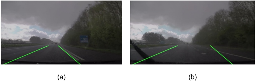
Fig. 13. (a)The frame in this figure shows the maximum IOU of 84.25% (b)The frame in this figure shows the minimum IOU of 61.38%
