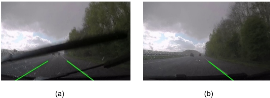
Fig. 9. (a)The frame in this figure shows the maximum IOU of 96.46% (b)The frame in this figure is the first frame and it shows the minimum IOU of 0%
