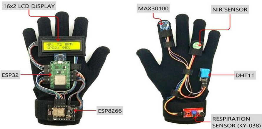
Fig. 2. Hardware prototype of the SmartLife Guardian monitoring System.
