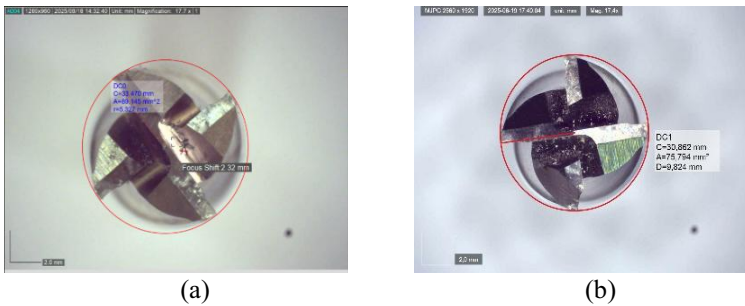
Fig. 8. Condition tool wear (a) before and (b) after
