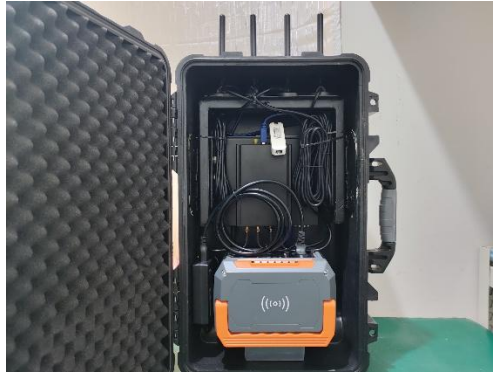
Fig. 2. Physical setup of the proposed private LTE system.
