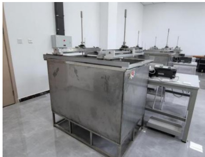
Fig. 3. Stainless Steel Experimental Water Tank
