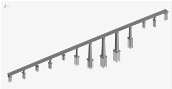
Fig. 2. A model of high-speed railway bridge under construction
