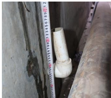
Fig. 4. Leak hole layout under upward leakage condition.
