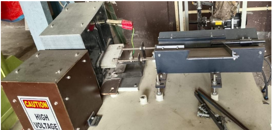
Fig 3. Typical industrial induction billet heating system (75 kW, 10 kHz), commonly used in forging and heat-treatment applications
