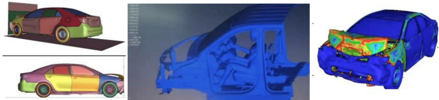
Fig. 14. LS-DYNA simulation deformation diagram
