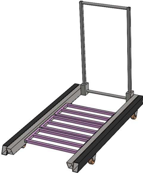
Fig. 1. CAD model trolley setup.
