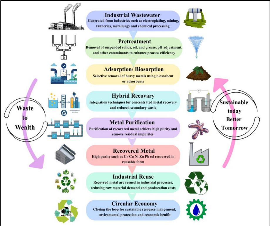
Fig 3. Schematic illustration of the integrated waste-to-wealth approach for sustainable heavy metal recovery and industrial wastewater reuse within a circular economy framework
