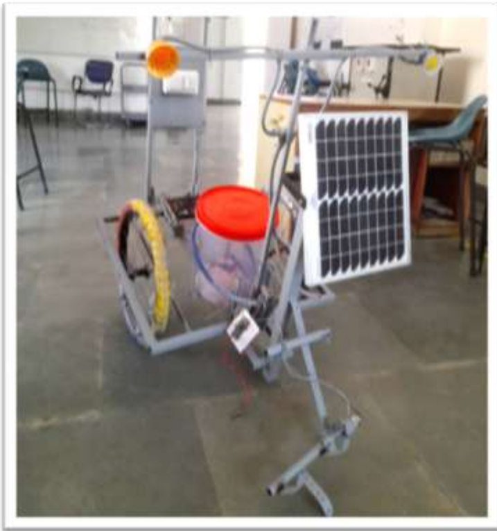
Fig.3 Final design of multipurpose solar-powered agriculture machine
