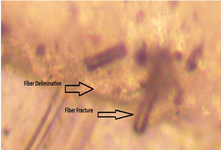
Figure 7. Image of fracture surface by using under optical microscope of tensile tests for transverse fiber unidirectional orientation
