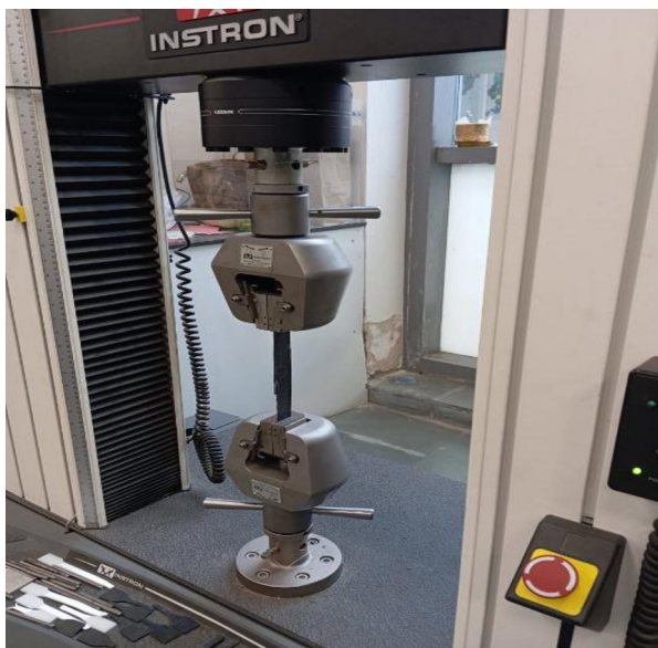
Figure 4. INSTRON Universal Testing Machine UTM 100kN with transverse unidirectional carbon fiber specimen.
