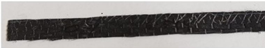
Figure. 2 A rectangular shape specimen having 90° orientation
