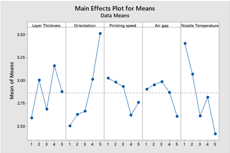
Fig. 3Main effect plot of Percentage error in linear dimension
