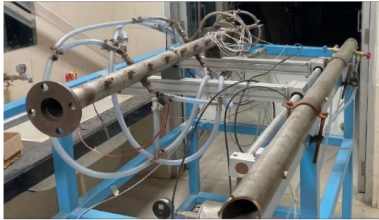
Fig. 1. Pulse Detonation Engine Setup at PEC.
