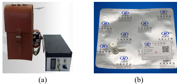
Fig.1. Gas sampling instruments: (a) Gas sampler; (b) Sampling bags.
