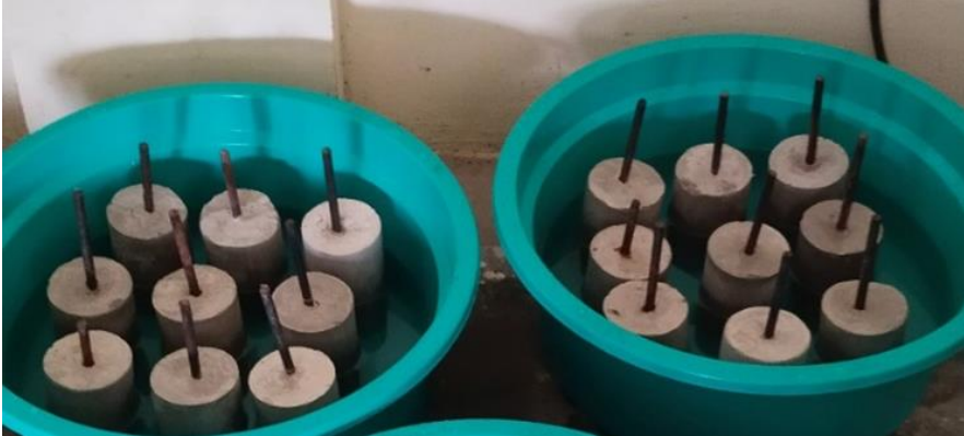
Figure 2. Visual appearance of the specimen immersed in artificial seawater
