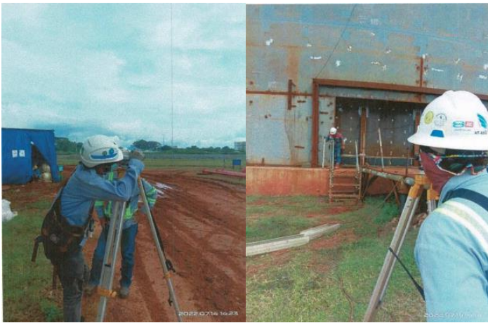
Fig. 3. Theodolite measurement on to the propane storage tank T-201
