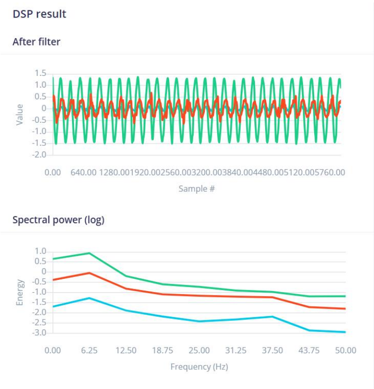
Fig. 9. Spectral plot of the normal motor shaft
