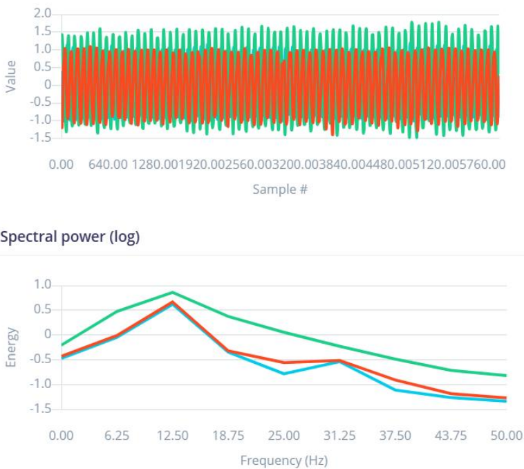
Fig. 10. Vibration plot of the bent motor shaft
