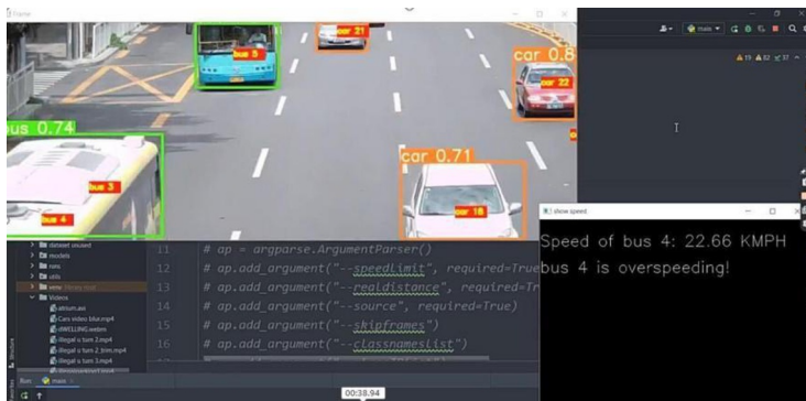
Fig. 7. Speed Violation Detection
