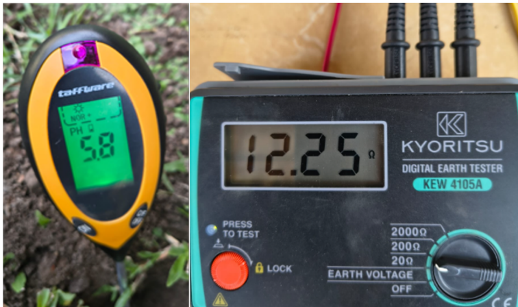
Figure 3. pH and Grounding Resistance before Eco-Enzyme Treatment
