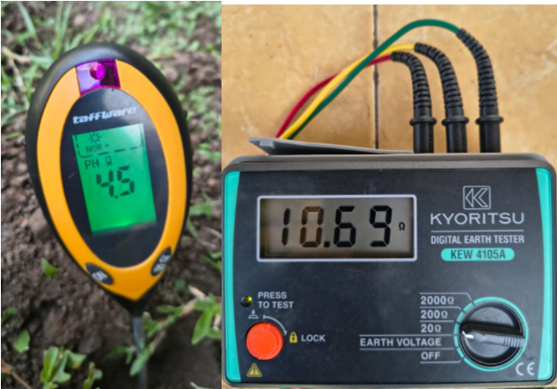
Figure 4. pH and Grounding Resistance after Eco-Enzyme
