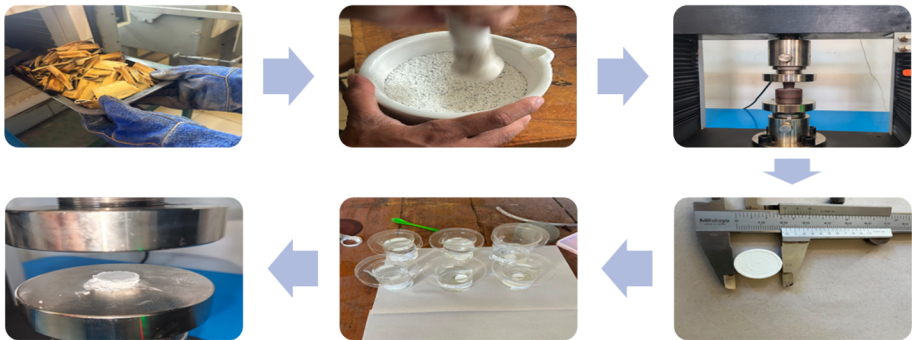
Figure 1. Experimental workflow illustrating the preparation of bovine bone-derived hydroxyapatite pellets, chemical exposure in different pH environments, and mechanical integrity evaluation.
