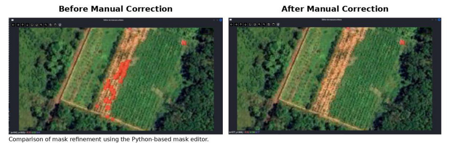
Fig. 3. Manual mask refinement using the Python-based correction tool.
