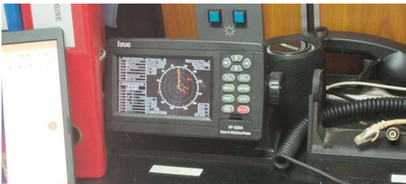
Figure 5. AIS (Automatic Identification System), one of the communication devices on board the Training Ship Barombong
