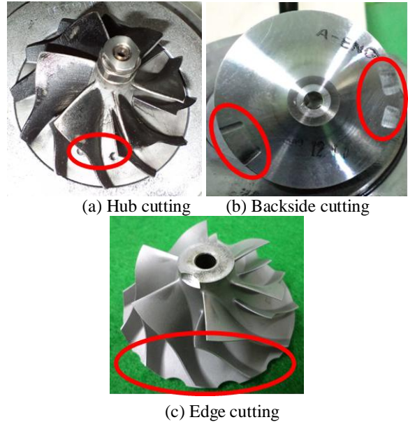
“Figure .2” Balancing methods compressor wheel
