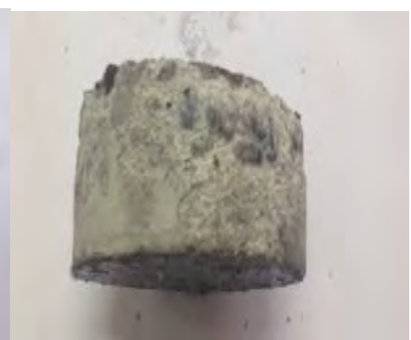
(c) Specimen after 40 freeze-thaw cycles
