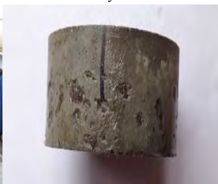
(b) Specimen after 10 freeze-thaw cycles
