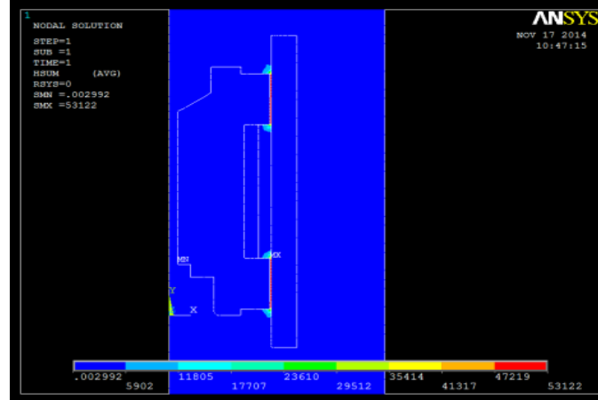
Fig.5 Distribution Contour of Magnetic field Intensity Simulation Result
