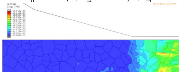
(a) Mises stress distribution when rolling process begin
