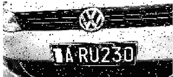
Fig.2 Enhanced image by histogram equalization
