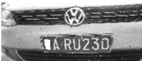
Fig.3 Enhanced image by median filter
