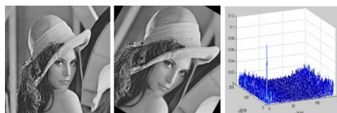
Fig. 3 (a) Images and phase correlation peak of frequency spectrum in log-polar coordinate
