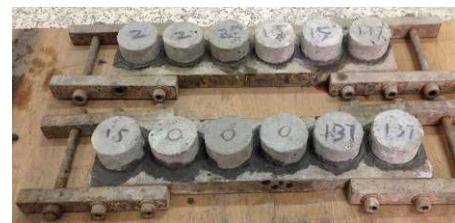
Fig. 3. Specimen of PVA- ECC
