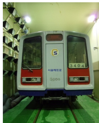
Fig.1: A subway cabin in a climatic chamber for the experiment
