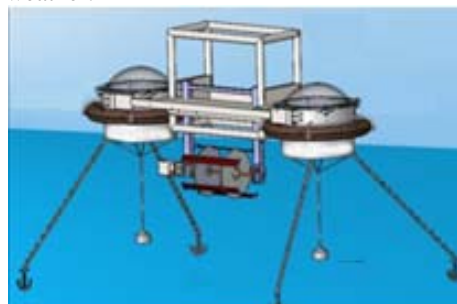
Figure 1. Generating system overall design
