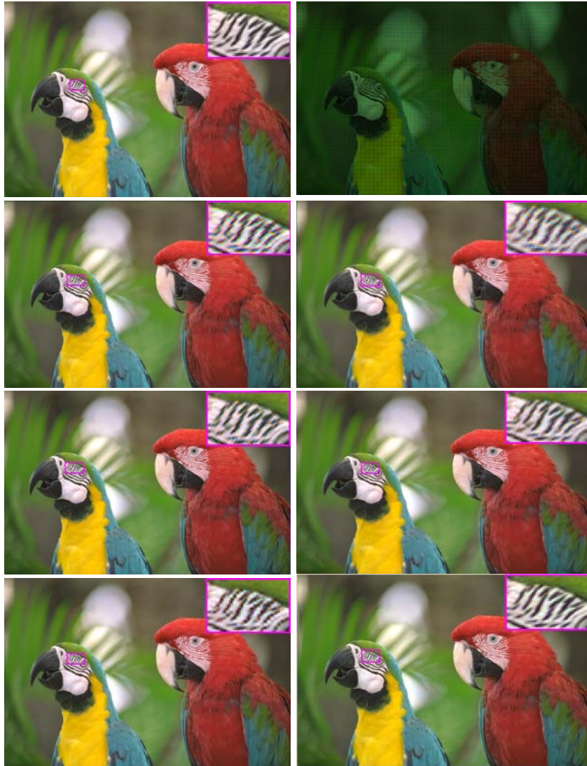
Fig.4. comparison of the Original and demosaicked results of parrots. From the first image to the last image: Original image, Bayer image, Nearest image, Bilinear image, Cok image, Laroche image, Hamilton image, Proposed image.
