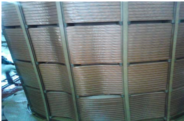
a. Low voltage side c phase winding deformation is most serious
