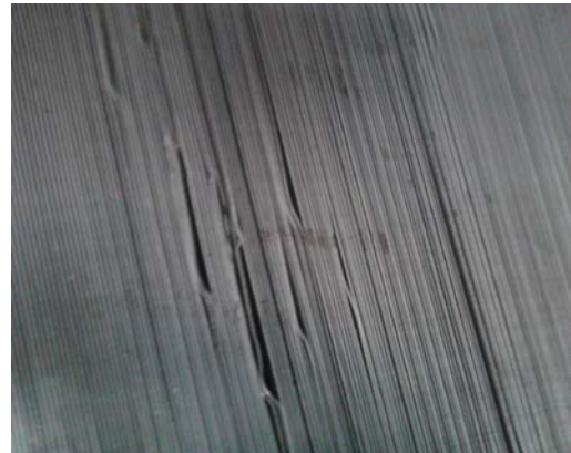
b. Iron core structure instability and deformation
