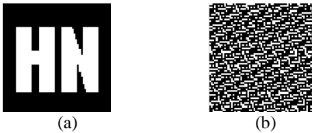
Figure1. The scrambled watermarking image using Arnold scrambling: (a) the original watermarking; (b) the scrambled watermarking.
