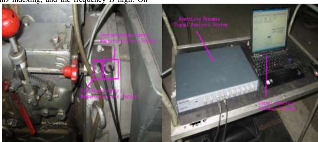
Figure 1. composition of instantaneous speed test system
