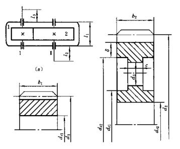
Figure 1. single stage cylindrical gear reducer
