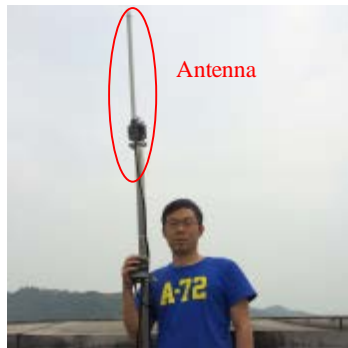
(a) ADS-B ground antenna
