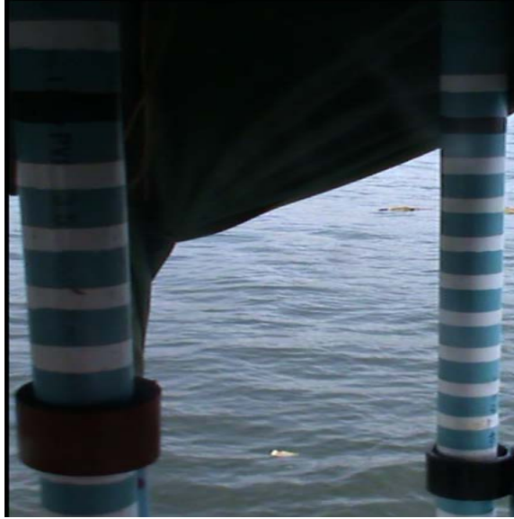
FIGURE II. THE EQUIPMENT FOR MEASURING WAVES (RIGHT) AND FLOATING BUOYANCY HEIGHT (LEFT).
