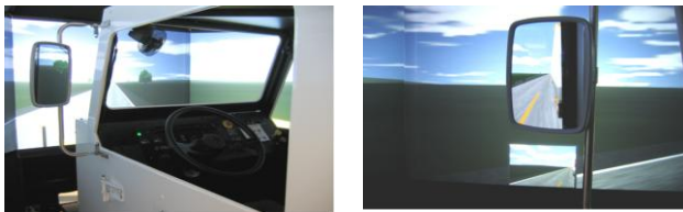
FIGURE I. THE TT-2000-V7 DRIVING SIMULATOR (LEFT) AND THE REAR VISUAL CHANNEL AS VIEWED THROUGH THE SIMULATOR MIRRORS (RIGHT).
