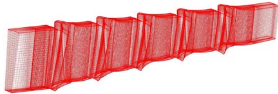
Fig. 2 Computational grid of 5-stage axial compressor
