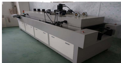
(a) WPCB disassembly equipment
