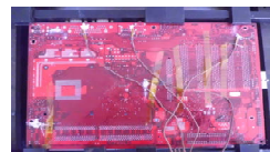
(c) Collect the surface temperature of PCB
